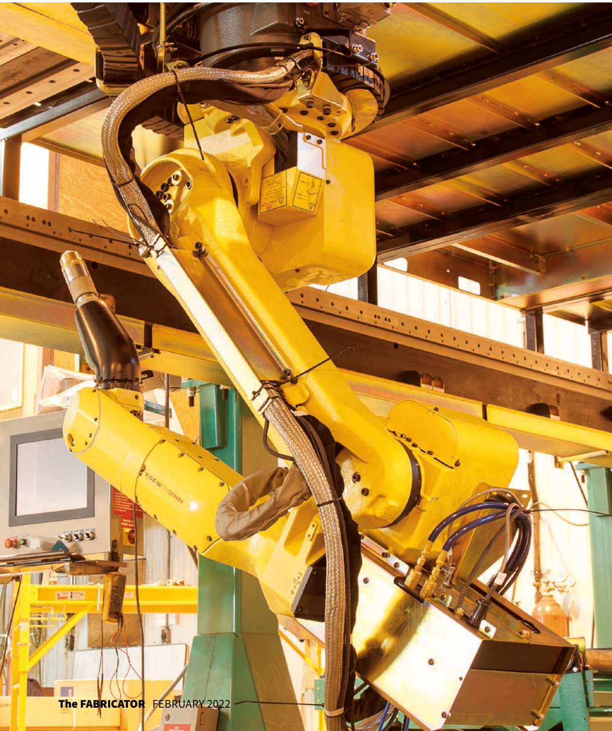
FIGURE 1 A standard torch body is designed for plate cutting. Using this same torch in multiaxis applications increases the chance of collisions with the workpiece.
